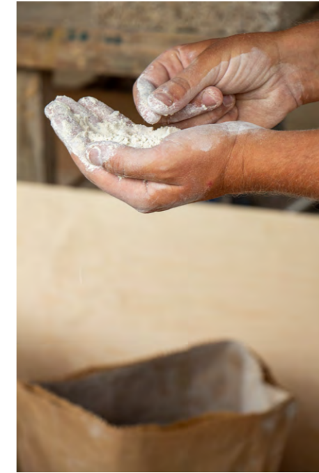
Léém Clay Paint is delivered as a fine dry mixture of clay and local mineral materials
