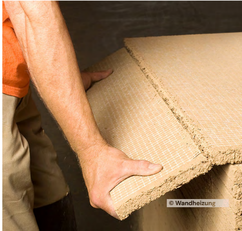
Earth panels are drywall panels that are screwed on a framework
