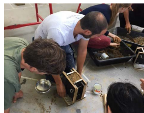
Step 1: place the mould on the ground and fill it with soil.
