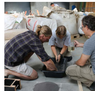
Mix well the soil with water to achieve humid and plastic states.
