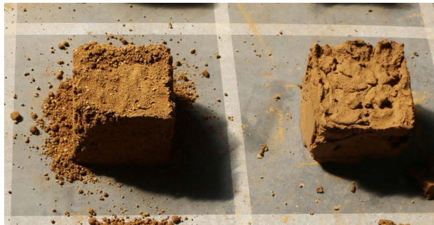
Tamped soil at humid state. (suitable for earth blocks production)
