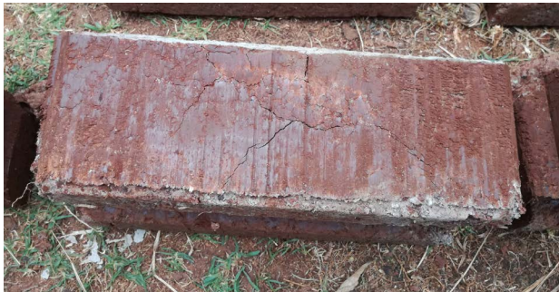
Clay soil presenting cracks due to shrinking
