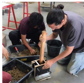
Step 4: compact well the soil with the help of a wooden stick.
